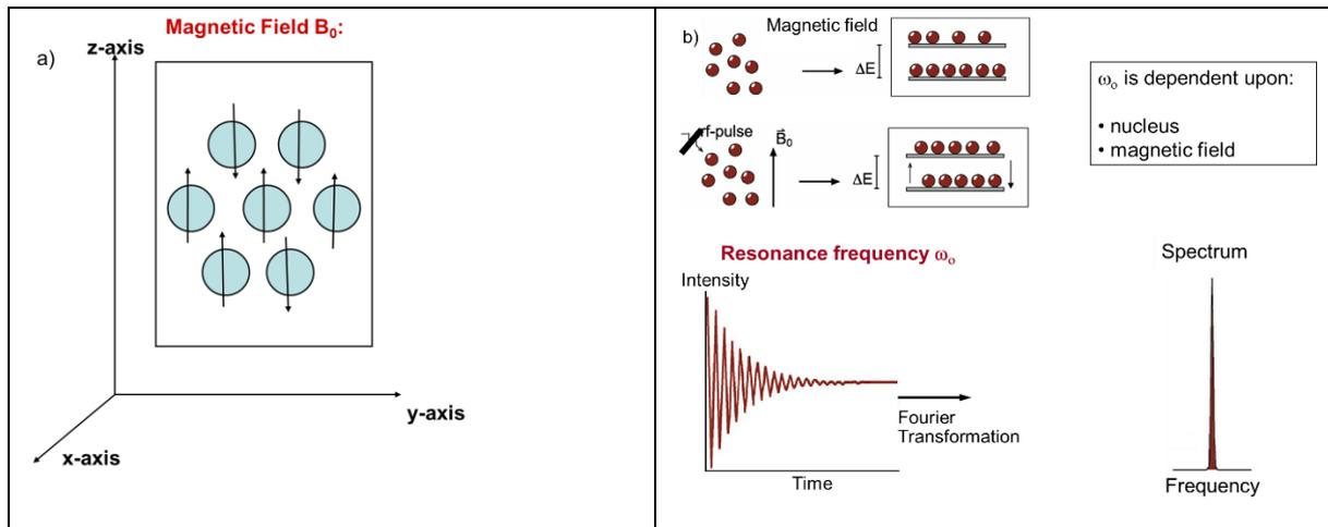
Figure 1: a) Nuclear dipoles in an external magnetic Field. b) the resonance condition (adapted from Knicker (2011))
